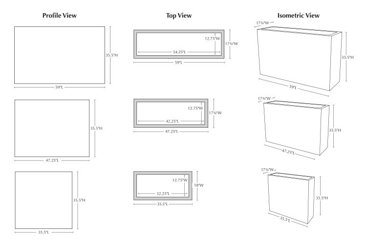
Materials: unsaturated polyester resin, sand, stone powder, talc powder, and fiberglass
