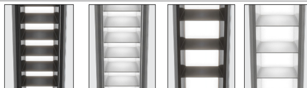
Black narrow micro louver shown - 60°, flush.
