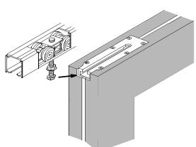
Track must be mounted securely to framing or blocking with #8 pan head screws at least 1-1/2" long. Track must be level even if floor and ceiling are not. Panels can weigh up to 150 lbs. apiece - reinforcement may be necessary. It is the responsibility of the installing contractor to determine. Longer spans will require lengths of track to be fit end to end - be sure both factory edges meet and align carefully. Track has 5.5mm holes every 12" and 2" in from both ends of track.
