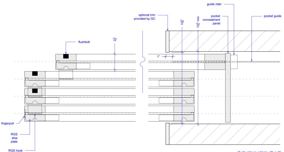
Guide rider is a block with a slit for the pocket guide; it allows for full extension, attach to bottom of concealment panel.
