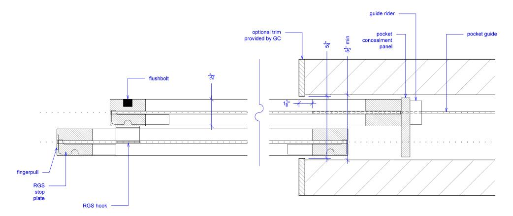
Guide rider is a block with a slit for the pocket guide; it allows for full extension, attach to bottom of concealment panel.
