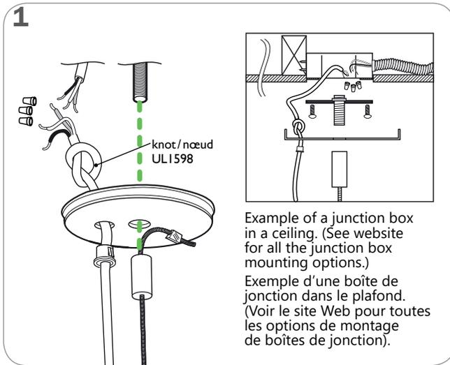
Connect the power cord to the ceiling power feed.
