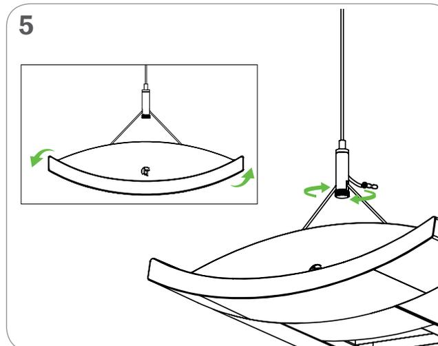
Partially unscrew the security screw and level the fixture straight.
