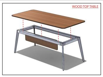
For Tables with wood tops, align through holes in top of rail with threaded inserts located in top. Secure with 1/4"-20 x 7/8" Joiner Bolts.
