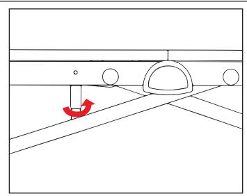
Tuning the flatness of the top can be done by rotating the screw as shown.
