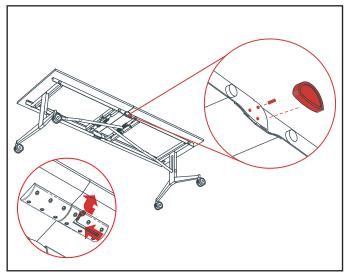
Ensure both lock latches are in the locked position and with the help of another person, rotate table onto casters. Remove blocking pin and replace cover cap.
