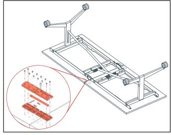
Assemble lock latch by aligning bottom housings, center pin, locking pin, lock throw, latch and top housing as shown. Fix housings to top with #8 x 1" wood screws. Repeat both sides.
