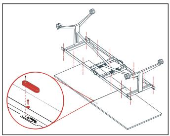
Place top sections face down on a protective surface, align through holes in frame with threaded inserts in top. Secure with M6 button head screws and washers. Note, slight movement of top and frame is required for anti-pinch feature. Install plastic cover & fix with #6 x 3/8" wood screw.
