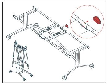
With the help of another person, carefully open the frame and insert blocking pin. This locks the frame into an open position and is critical to safe assembly.
