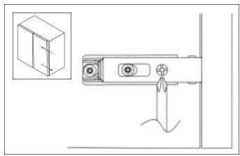
Adjusting this screw moves the door sideways to adjust the gap between doors (minus 0.5 mm to plus 5.0 mm).
