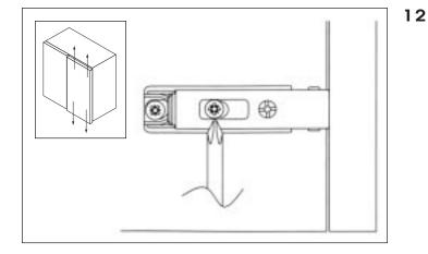
• Adjusting this screw moves the door vertically (plus or minus 2.0 mm).
