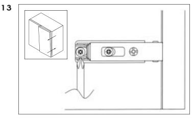
Adjusting this screw moves the door in or out from the cabinet (minus 0.5 mm to plus 2.8 mm).
