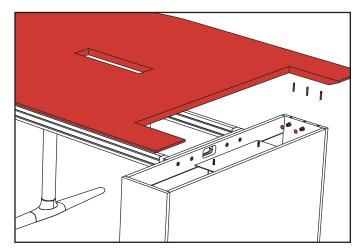
Insert mini-fix cams into rebated holes inside of media case. With top upside down on a protective surface, install mini-fix posts in bottom of top. Rotate top, align posts with holes in top of case and set in place.
