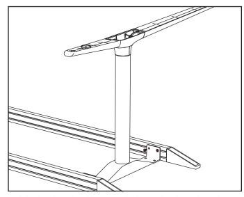
With both rails and end base upside down, align base through holes with pre-installed rail t-slot nuts and fix with 1/4"- $20 \times 9/16$ " joiner bolts.
