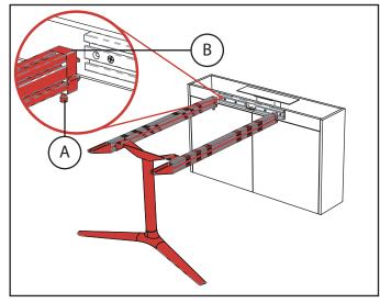
Loosen gripper socket head screws (A). Rotate base / rail assembly and align gripper fitting (B) with mounting profile. Position assembly centered on case and tighten gripper screws to lock.
