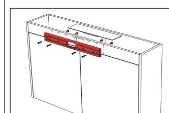
Align through holes in rail mounting profile with corresponding holes in media case and lock plate. Secure with  $1/4''-20 \times 1 \ 1/2''$  flat head bolts and joiner nuts.
