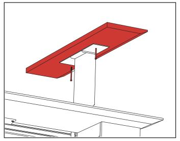
The lift lid is installed by aligning threaded inserts with through holes in TV bracket. Secure with 1/4"-20 x 3" socket head screw. Note, the lid is meant to be loose. This is to ensure fingers are not pinched during operation-see lift guide for further safety features.
