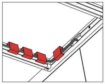
Wiring is routed to the media case with "U" clips that install to both rail and mounting profile.
