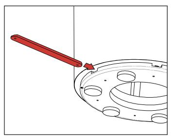
Ganging elements together is achieved by inserting either 6 1/2" or 9 1/2" ganging clip with angled portion facing up, into slots in base. An audible click will be heard once clip is locked into position.
