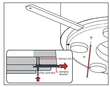
To unlock, insert Tite-Joint Rod into small hole nearest the ganging clip. Depress spring lock while gently pulling the ganging clip away.
