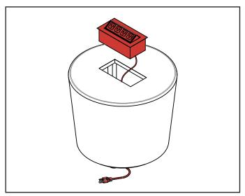
To install Power / Connectivity device follow instructions included with your specific device. Wiring exits the element through 8"dia. hole in bottom.
