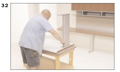
• Install leg to return bottom with machine screws.
