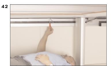
• Remove the small machine screw that is inside the dimmer switch under the top. Place the small cable inside the dimmer switch and re-insert the screw. Tighten.
