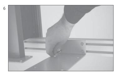
• Attach the support bracket to the rail using 9/16" x 1/4"-20 flat head hex socket bolts (8 per bracket).
