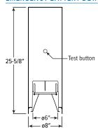
Test button is located in the cylinder side wall, standard.
