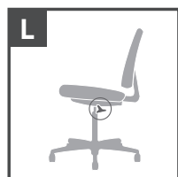
L. Tilt lock — Locks out tilt function.
