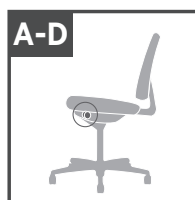
A-D. Side tilt tension — Controls rate and ease of recline. Conveniently located on the right side.
