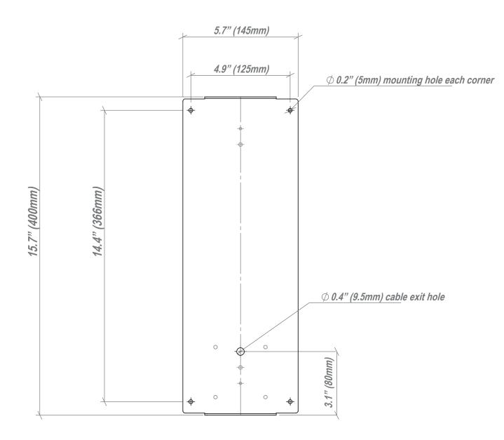
Backplates can be rotated 180 degrees- to allow cable exit to be positioned at top if required.
