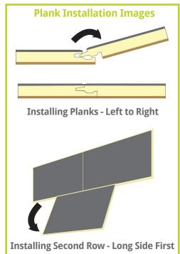
Use a thumb, finger or hand to set the locking mechanism and ensure that planks are aligned - if necessary, use a straight edge, level or equivalent to ensure top edges are flush. Use a 16 oz. rubber or poly-based dead blow hammer or a #2 rubber mallet to lightly tap and lock planks completely into place. **Do** not use a hammer or tap directly on the seam/locking mechanism, as this could cause permanent damage to the locking mechanism.
