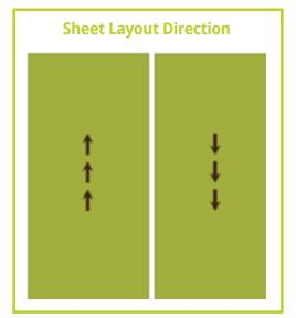
Once seam location is established, layout and rough cut sheets from the roll - allow for 3" - 6" of excess material. Rolls should be laid out and installed in sequence, following the numeric order of the rolls. When cutting sheets from a roll, be sure to turn every other sheet by 180° so that sheets are alternating in direction.
