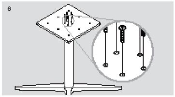
Use five 1/4-20 x  $3/4^{\circ}$  button socket cap bolts in a staggered procedure until all of the bolts are tight.
