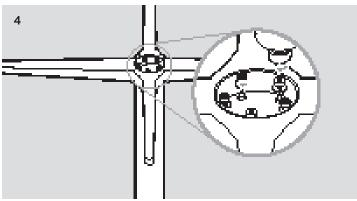
Tighten bolts using a staggered procedure until all of the bolts are tight.
