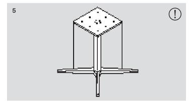
Assemble the mounting plate to the column. The corner of the plate must line up with the leg.
