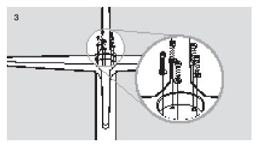
Line up the holes and assemble using the five 1/4-20 x  $1^{3/4}$  socket head cap bolts and lock washers.
