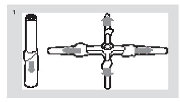
Peel back protective polyfoam on both column and base.
