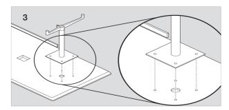
Line up the second base plate with the 4 screw inserts on the underside of the table top.
