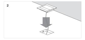
Feed the power cord through the center of the table top and fit the power box into the cut out.
