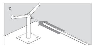
Slide the crossbar extrusion over the base insert, but do not secure.
