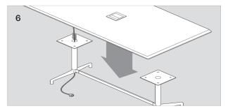
Before the connected base is fastened to the table top, feed the cord through the leg and out the bottom of the base.
