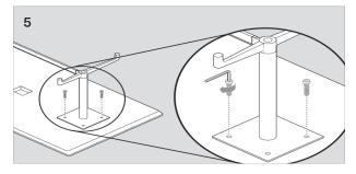
Lightly fasten (2)  $1/4 - 20 \times 5/8$ " screws with a hex key to secure the second base to the top.
