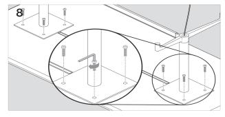
Ensure the base plates are lined up properly to the holes on the underside of the table and use the (8) 1/4 - 20 x 5/8° screws to secure the base to the top.
