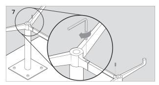
Secure the cross bar extrusion by fastening the (2) 5/16 -  $18 \times 1^{\circ}$  set screws with a hex key or driver gun.
