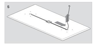
Depending on the location of the power source, run the power cord through the appropriate channel of the plastic cord management piece.
