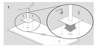
Line up the first base plate with the 4 screw inserts. Lightly fasten (2)  $1/4 - 20 \times 5/8^{\circ}$  set screws to opposite corners with a hex key.
