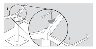
Connect the 2 halves of the base together with the crossbar extrusion using the (2)  $5/16 - 18 \times 1^{\circ}$  set screws, but do not fasten the base to the top.
