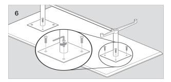
Fasten both base plates to the table top with the remaining (4) 1/4 -  $20 \times 5/8^{\circ}$  screws using a hex key or driver gun.
