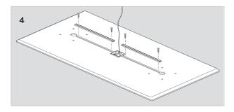
Fasten the 2 plastic cord management pieces into the corresponding channels using 4 wood screws.
