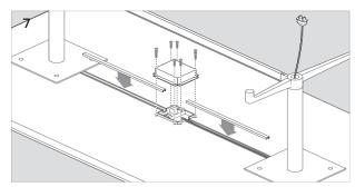
To hide the power box and cord, screw the power enclosure over the power box using the (8) 1/4 - 20 x 1/2" screws, and clip the smaller plastic cord management pce over the cord into the channel.
