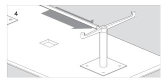
Slide in the cross bar extrusion to the second base to connect the structure, but do not secure.
