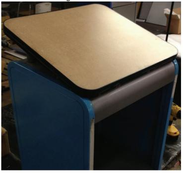
**Step 4:** Attach the Top to the cascade unit by using the 1.25" bolts on the rear with the poles, and the 0.5" bolts on the front with the brackets. Be sure to use the washers on the inside of the unit, when attaching the bolts from underneath.
