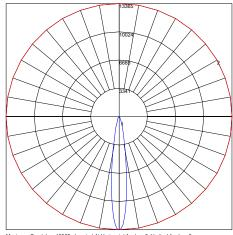
Maximum Candela = 13365 Located At Horizontal Angle = 0, Vertical Angle = 0 # 1 - Vertical Plane Through Horizontal Angles (0 - 180) (Through Max. Cd.) # 2 - Horizontal Cone Through Vertical Angle (0) (Through Max. Cd.)
