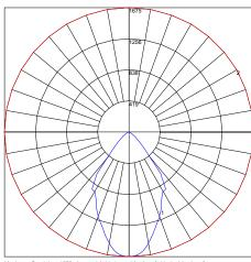
Maximum Candela = 1675 Located At Horizontal Angle = 0, Vertical Angle = 0 # 1 - Vertical Plane Through Horizontal Angles (0 - 180) (Through Max. Cd.) # 2 - Horizontal Cone Through Vertical Angle (0) (Through Max. Cd.)
