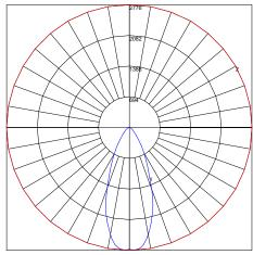
Maximum Candela = 2776 Located At Horizontal Angle = 0, Vertical Angle = 3 # 1 - Vertical Plane Through Horizontal Angles (0 - 180) (Through Max. Cd.) # 2 - Horizontal Cone Through Vertical Angle (3) (Through Max. Cd.)
