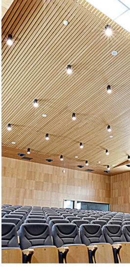
WoodLine Parallel wall and ceiling planks feature a continuous linear aesthetic utilizing straight lines. Planks are available in genuine wood veneer or laminate, with a reveal or flush edge. Reveal edges include an acoustical textile, providing additional performance. Flush edges leave a 5/64" space between planks. Perforations can be added to Parallel wall and ceiling planks to achieve optimum acoustical results.
