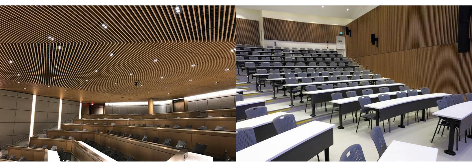
WoodLine Slat is a traditional linear wall and ceiling system that incorporates various blade sizes and spacing. WoodLine Slat is available in 1' wide by 8' long sections, with arrangements of three to eight blades per section. Sections are installed using an attachment clip suspended from a heavy duty 15/16" T-grid, and work with both backer and dowel assemblies. Available in genuine wood veneer or laminate. Various acoustical materials can be utilized to garner different acoustical results.
