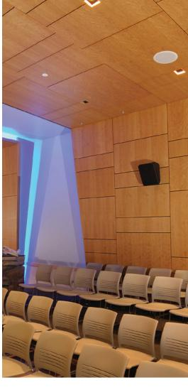
WoodLine Classic wall and ceiling panels are installed using pivot clips into a standard 15/16" T-grid. Panels are available in genuine wood veneer or laminate, with a reveal or flush edge. Reveal edge panels leave a 3/8" space between planks; wood strips are provided to conceal the pivot clip. Flush edge panels fit together seamlessly, creating a 5/64" bevel detail. Perforations can be added to Classic wall and ceiling panels to achieve optimum acoustical results.
