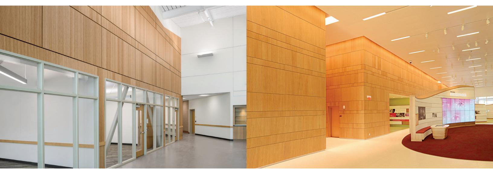
WoodLine Groove wall and ceiling planks allow for a wide range of acoustical performance through various width and spacing configurations. Installation is simple by utilizing a unique tongue and groove system, designed to work in conjunction with a 5/0 nailclip, creating an overall monolithic appearance. Groove panels are available in genuine wood veneer or laminate; perforations can be added to achieve optimum acoustical results.
