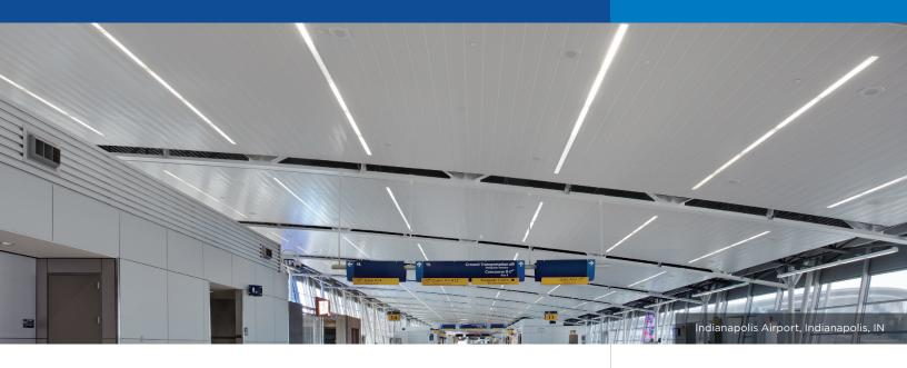
300C metal ceiling panels offer a subtle, long span design for interior ceilings. This panel features a butt-joint, "bevel edge" that moderates panel-to-panel connections for an orderly, finished design.
