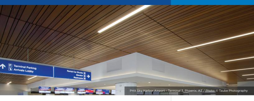
The Multi-Box Continuous metal ceiling system uses a universal carrier enabling an unlimited combination of panel depths and widths using Box and Deep Box 2", 4", 6" and 8" panels.
