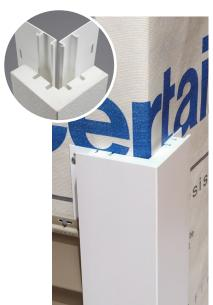
alternative to traditional face nailing. Trimboards and J-Pocket Trimboards feature grooved millwork that precision-fits to flanges secured directly to the wall, working together with both nail hem flange and starter flange for a secure fit. The flanges are concealed, leaving a face nail-free installation with no nail holes to fill. One-piece corners also utilize the same nail hem flange, eliminating the need to face-nail.
