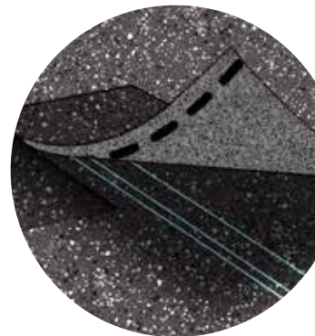
Diagram for illustrative purposes only. Ceramic coating Mineral core Copper layer
