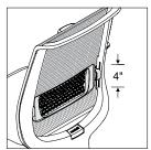
**Lumbar height** adjusts 4" (6" to 10" from seat) by grabbing exposed tabs and sliding the lumbar support up or down. Available as an option on mesh work chairs only.
