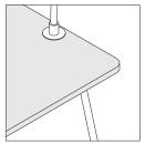
**Verb teaching station worksurfaces** are woodcore with High-Pressure Laminate top and plastic 3 mm edge band.
