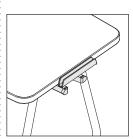
**Side docks** allow display of whiteboards on the tables. For best results, rock the boards into place rather than pressing straight down. Side hooks allow storage of up to four boards per hook. Tip: Side docks are not available on 19"D personal tables with casters.
