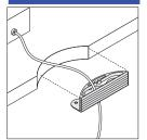
Worksurface wire managers are available to convert cable scallops into grommets in freestanding applications. They are included with wood veneer worksurfaces. Wire managers can be used with Universal worksurfaces.
