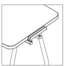
**Side docks** allow display of whiteboards on the tables. For best results, rock the boards into place rather than pressing straight down. Side hooks allow storage of up to four boards per hook.
