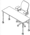
Standing-height adjustable legs adjust on 1" increments from 28½"–45" (includes top thickness). The legs measure 24"–40½" with 3¾s" levelers. Due to the large range of the leveler, tables may vary in height depending on how far the leveler is inserted into the leg. The 1" adjustments match the Kick Systems vertical upright adjustment pattern.
