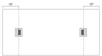
For the power option with both ends, the centerline of each power module is located 10" from the short edge of the table. Power module flips toward the center of the top.
