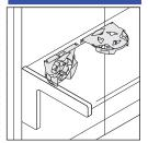
Reel can be field installed vertically or horizontally in the kneespace of freestanding desks or panelsupported worksurfaces.
