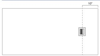
For the power option with one end only, the centerline of the power module is located 10" from the short edge of the table. Power module flips toward the center of the top.
