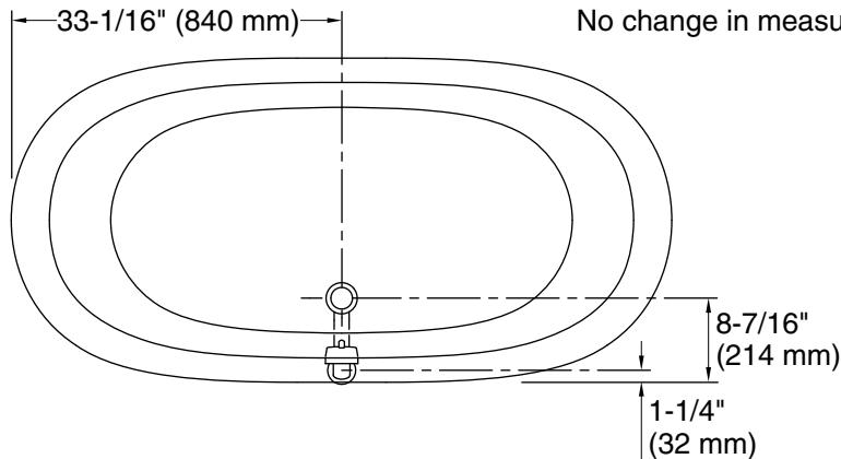
No change in measurements if connected with drain illustrated. (K-7159)
