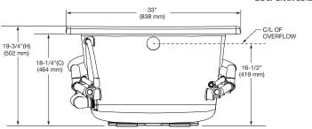
■ DIMENSIONS OF FIXTURES ARE NOMINAL AND MAY VARY WITHIN THE RANGE OF TOLERANCES ESTABLISHED BY ANSI STANDARDS Z124.1 AND A112.19.7.
