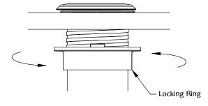
Screw threaded lock ring onto mounting collar by turning clockwise. Locking ring should rotate smoothly once properly engaged. If not, the locking ring may be cross-threaded - undo and try again.
