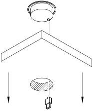
Install the unit into the cut out and be sure it is fully level on the surface. Use of adhesive is recommended for a more secure fitting (Not included).
