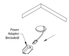
Plug in the USB cord from the unit to the power adapter. Plug the power adapter into a nearby outlet (outlet should be close enough to where power cord is not taut or strained) and unit is ready for use.
