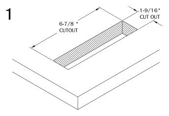
Make a cut out on the desired surface. (Note: Maximum corner radius 1/8".)
