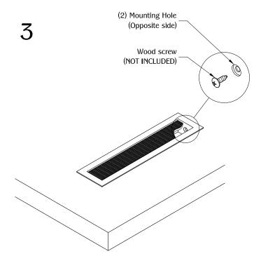
Use (2) Wood screws through the MAX11B mounting holes to secure on to the table top.
