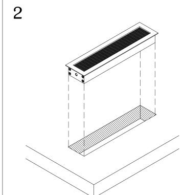
Install MAX11B into the cut out and be sure it is fully leveled onto worksurface.
