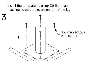
Use (4) flat head mounting screws to secure the part onto the work surface. (Note: Use appropriate screws and screw length depending on the table type and thickness.)
