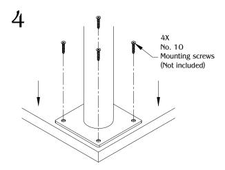
Secure the leg by using (4) No. 10 mounting screws. (Note: Use appropriate screws and screw length depending on the table type and thickness.)
