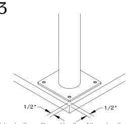
Determine the position and location of the part on the work surface. Allow  $1/2\,{}''$  clearance at the edge of the work surface.
