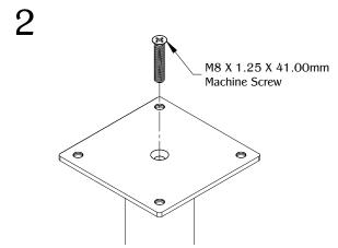
Secure the TP/5" SQ to the TL76 by tightening the M8 X 1.25 X 41.00mm machine screw.
