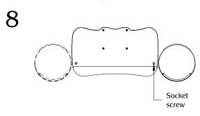
Remove the socket screw with a 4mm Allen wrench (NOT INCLUDED). Install the mouse pad at the pre-drilled countersunk hole at the bottom right or left tray for a left-handed or right-handed use.
