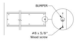
Mount the track on the underside of the work surface using (8) #8 wood screws.
