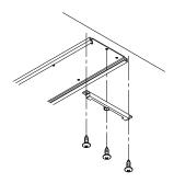
Slide the mechanism back to the bumper. Install the track guard at the front end of the track using (3) #8 wood screws.
