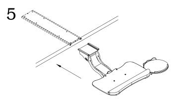
Slide the KP7 tray and mechanism into the mounted track.
