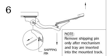
Tip front of the KP7 tray up and begin to lower mechanism to relieve pressure on the shipping pin. Pull out the shipping pin.
