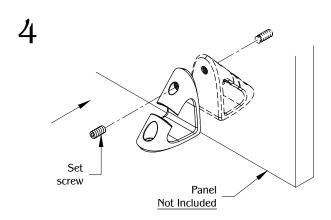
Place the panel material in between the PGRP9. Secure the panel with (2) set screws. (Note: 18" recommended maximum panel height.)
