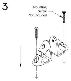
Align the PGRP9 to the pilot holes. Use (2) mounting screws and secure the part on top of the work surface.
