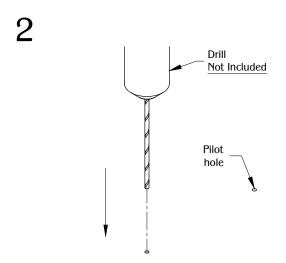
Drill (2) pilot holes to mount on the work surface.
