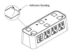
Peel off the adhesive backing on all six snap-in adhesive pads.
