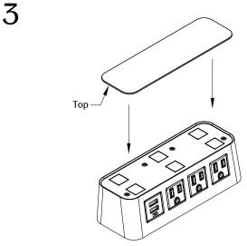
Align the top to the unit. Make sure it is fully leveled onto the top surface. Plug the unit into a nearby outlet and unit is ready for use.
