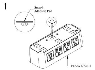
Determine the position and location of the unit on the work surface. DO NOT place unit where the cable is strained or trapped. Align the snap-in adhesive pads to the top of the unit.
