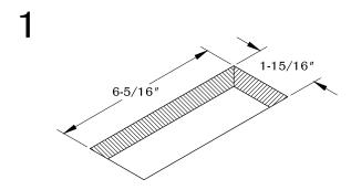
Make a cutout in the desired location on your work surface. Allow enough clearance for unit operation. DO NOT place unit where the cable is strained or trapped.
