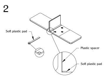
Place the spacer on the inside wall of the large panel grip. Peel the adhesive film off the soft plastic pad and stick next to the plastic spacer. Make sure it is centered.
