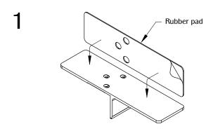
Peel the adhesive film off rubber pad and stick on to the bottom of the large panel grip. Make sure its centered.
