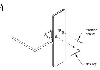
Squeeze panel grips and Secure the panel using (3) machine screws. Repeat steps as needed for additional panel grips.
