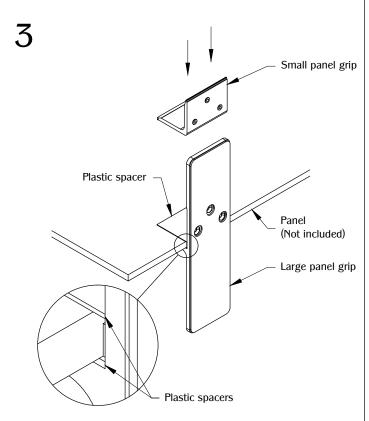
Place panel on work table, then place large panel grip on the bottom including plastic spacer (1 additional plastic spacer for use as needed). Then slide small panel grip from the top including plastic spacer.
