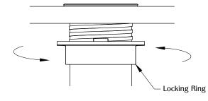
Guide the cord through the cut out. Install the unit into the cutout and make sure it is fully level on the surface.
