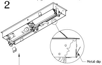
Place the metal clips near the front and back of each side of the unit. (NOTE: Metal clips are for use in hard surface material only as an optional mounting means.)
