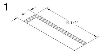
Determine the position and location of the unit on the work surface. Cut the hole at 16-1/4" X 4". Place and allow enough clearance for unit operation. DO NOT place unit where the cables are strained or trapped.
