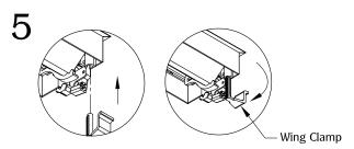
Secure unit by turning bottom wing clamp.
