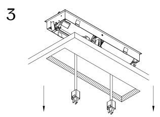
Guide the power cords through the cut out. Install the unit into the cut out and make sure it is fully leveled onto the surface.
