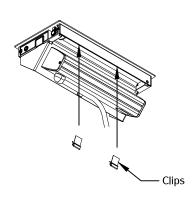
Install the clips at the back of the unit.
