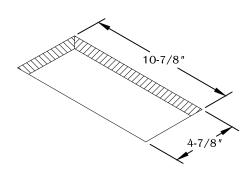
Determine the position and location of the unit on the work surface. Place and allow enough clearance for unit operation. DO NOT place unit where the cable is strained or trapped. Cut the hole at 10-7/8" X 4-7/8".
