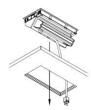
Guide the power cord through the cut out. Install the unit into the cut out and make sure it is fully leveled onto the surface. Plug the unit into nearby outlet and unit is ready for use.
