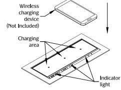
Position the mobile device on the center of the charging area. The indicator light activates to signify that the device is actively charging or the charging icon will activate on the device's screen.
