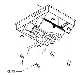
Place clips before installing in cut out.
