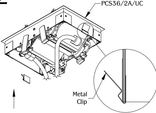
Place metal clips near the ends of the front and back of the unit. (NOTE: Metal clips are for use in hard surface material only as an optional mounting means.)
