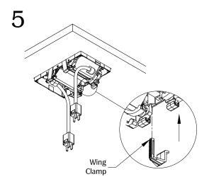
Secure unit by turning bottom wing clamp.
