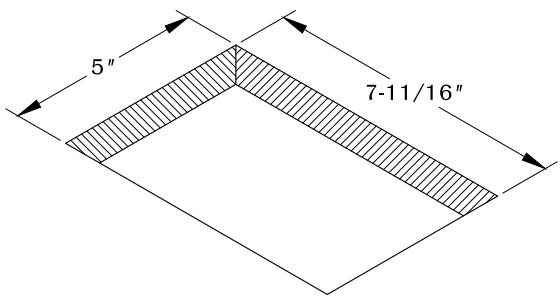
Determine the position and location of the unit in the work surface. Cut the hole at 7-11/16" X 5". Place and allow enough clearance for unit operation. DO NOT place unit where the cables are strained or trapped.
