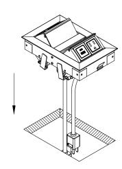
Guide the power cords through the cutout. Install the unit into the cutout and make sure it is fully leveled onto the surface.
