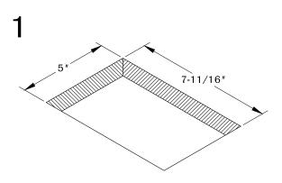
Determine the position and location of the unit in the work surface. Cut the hole at 7-11/16" X 5". Place and allow enough clearance for unit operation. DO NOT place unit where the cables are strained or trapped.
