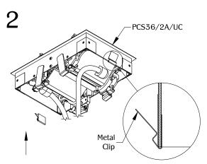
Place metal clips near the ends of the front and back of the unit. (NOTE: Metal clips are for use in hard surface material only as an optional mounting means.)
