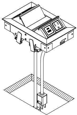
Guide the power cords through the cutout. Install the unit into the cutout and make sure it is fully leveled onto the surface.
