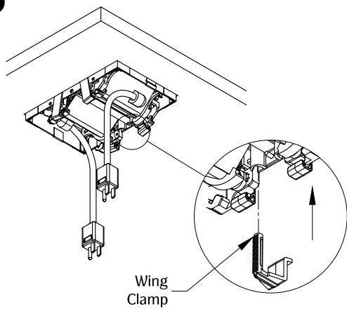
Secure unit by turning bottom wing clamp.
