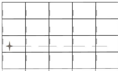
Diagram - End of Run *Power In-Feed and (4) Jumpers
