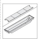
Power channels are available in the table top to provide lay-in cable routing and access to electrical outlets and voice and data receptacles. Technology covers are included to conceal outlets and receptacles. Tables can accommodate one or two power channels depending on table dimensions. Power channels are standard with a conduit and must be hardwired in the field.
