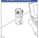
Power and communication spheres are field installed. You can specify a factory-cut mounting hole in Convene tables to accommodate spheres, or use a 3" diameter drill to cut mounting hole at desired location.
