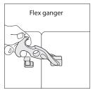
**Flex gangers** can be used to easily link adjacent tables in multiple configurations. Flex gangers use a flexible loop that engages a hook to hold two adjacent table tops in place. No tools are required to stretch the loop across the seam between two table edges and to connect it to the hook on the adjacent table. All flex ganger locations are pre-drilled for simple relocation when desired.
