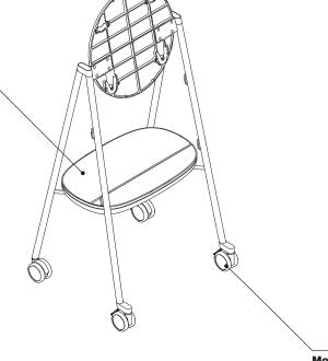
**Mobile stand** includes 360° rotating casters. Front casters are locking and back casters are non-locking.
